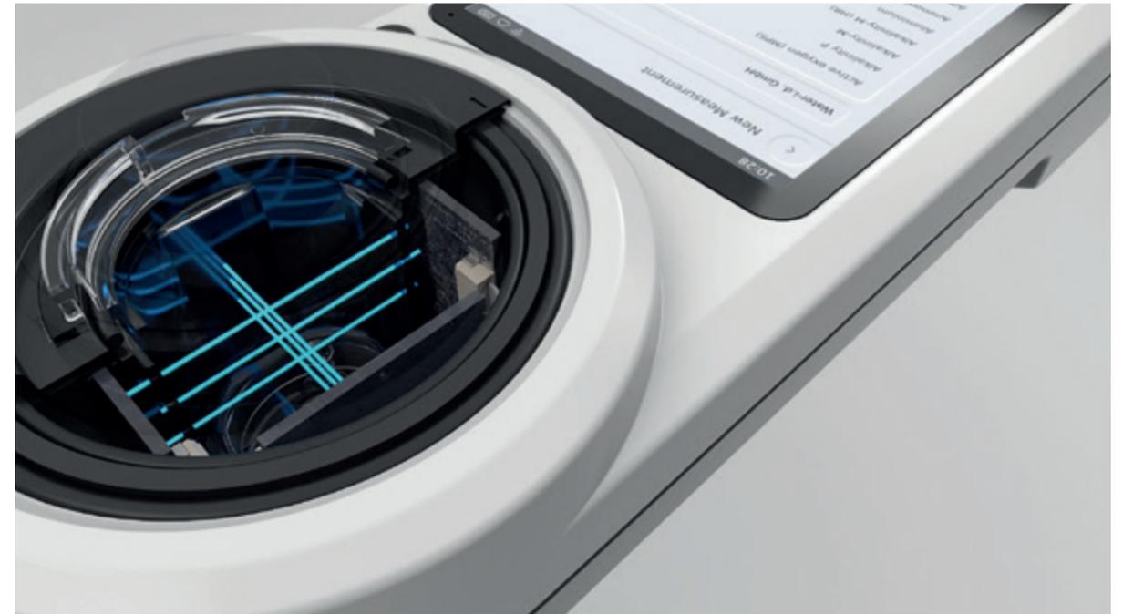
While normal photometers perform measurements on one selected wavelength only, the PrimeLab 2.0 can receive data from 18 different wavelengths, covering the key parts of UV and IR section of the spectrum and the full VIS range.
