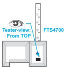
**5** Move the parameter stick to the last recognizable point and read the result next to the point.
