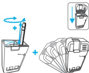
Remove the cap and place the parameter stick under the right measuring chamber.
